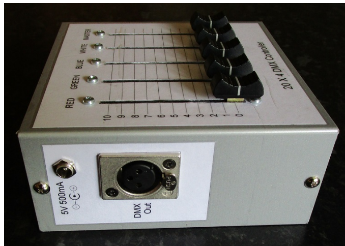
Illustration 4: Side view showing the power and DMX connections
