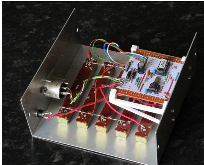
Illustration 3: Layout of components inside the enclosure
